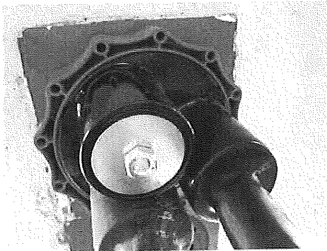
Illustration 20: HSI 150 D3/58 with seal plugs VS58/60, hot and cold shrink-on sleeve in HSI 150-K 100, trough under-side after 92 days
